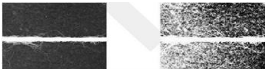
Fig.6-Image of yarn on black background and Resultant image after histogram equalization
