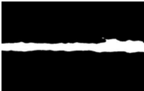
Fig.11- Binary image generated after thresholding at 0.4762
