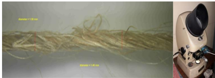
Fig.3 - Manual jute yarn diameter measurement using image
